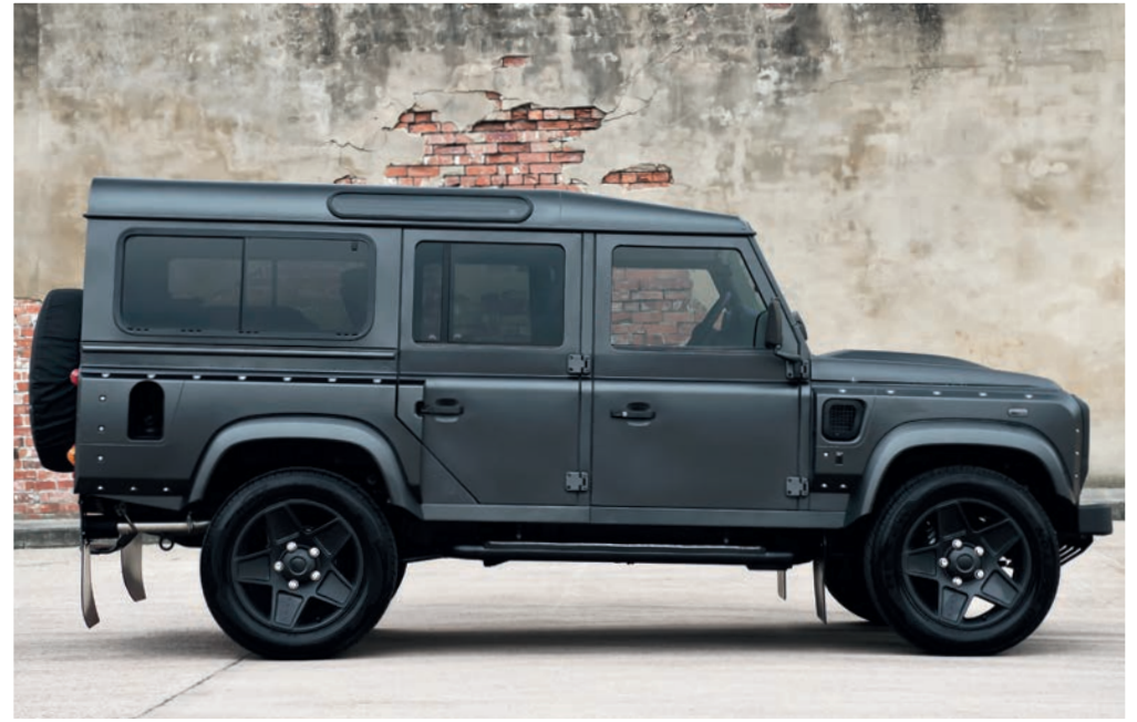
Front & Rear Wide Wings with Integrated Bolts & Apertures in Light Weight Composite Mounts onto the existing wings (Supplied in self-colour)
