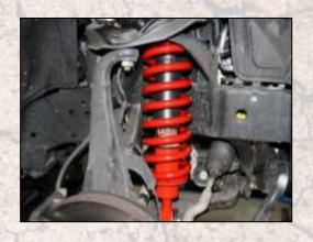
Terrafirma has teamed up with Pedders, World renowned Suspension manufacturers from Australia and now offers a range of Suspension upgrade kits for popular 4x4 pick-ups. Designed to provide a 40mm lift, improve the load carrying performance, ride comfort and appearance which allows for larger diameter tyres to be fitted. The kits are a complete engineered suspension solution for your pick up guaranteed to improve on road and off road handling and capability.
