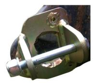
Ensure the rear axle is centralised in the rear wheel arch and then measure the distance from the centre of both mounting bracket holes to get the length your new adjustable arm needs to be. Make a note of this to ensure both sides are the same length.
