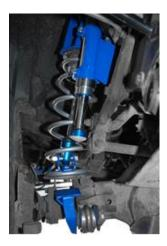
Fit the chassis plates with the vertical plate towards the back of the vehicle. Attach this using the two rear bolts only (M12x100 with washers) align the plate using the original bolts through the front holes and fully tighten the new rear bolts. Remove the front alignment bolts.
