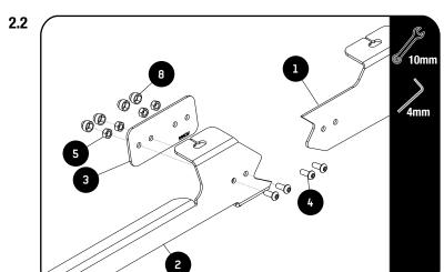
Assemble the Front and Rear Foot Rail (Item 1 & 2) together with the Joiner plate (Item 3)
