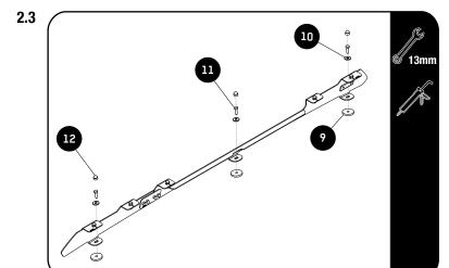
Put a small amount of silicone ove each Mounting Point and place the spacer (Item 9) on top of the silicone, lining up with the hole in the spacer with the mounting noint.
