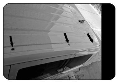
Starting by removing the 8 x OEM M8 screws from the roof.
