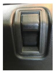
4. Remove the window winder handle by removing the "c" clip behind the cover -
