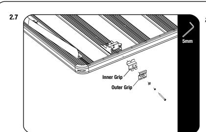
Loosley fit one Inner Grip and one Outer Grip to each Grab On Foot using a M6 Cap Screw, M6 Spring Washer and M6 Cap Screw Washer removed.
