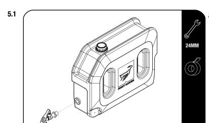
When fitting the tap, apply thread tape to the thread of the tap.
