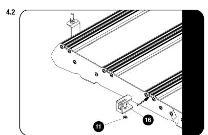
Assemble the M8 x 16 Button Head and M8 Thin Nut (Items 11 & 16) to the Rear Mount Bracket (Item 5).
