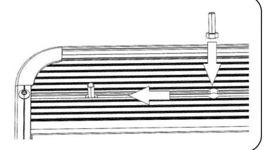
(B) With your rack still upside down from Step 3A, slide a M8 x 20 Hex Bolt (Item 5) into the end of Slats 2, 6, 7.
