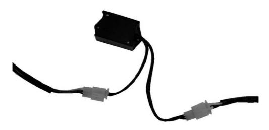
( C ) Reconnect the LED wiring harness to the vehicle's battery system. With the harness's switch in the ON position, the LED light may now be controlled via the remote control.
