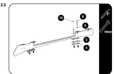
Place silicone over and around the jack nuts to create a watertight seal before placing the spacers over the jack nuts. Place the 6mm spacer (Item 4) onto the Jack nut.Place the 10mm Spacer (Item 3) on top of the 6mm Spacer (Item 4) As shown.
