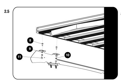
Assemble your roof rack to the Foot Rails using M8x20 hex bolts, M8x16x1.6SS Flat Washers and M8 Nyloc Nuts (Items 8, 9 & 10) as shown.
