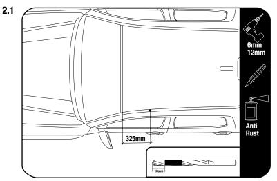
Starting at the top edge of the windscreen measure 325 mm along the ditch towards the rear of the vehicle. Mark the hole centre in the ditch as shown.
