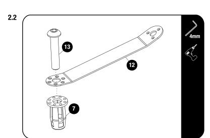
Insert a M6 x 30 Button Head Bolt (Item 13) into the Jack Nut Tool (Item 12) and loosely fit a Jack Nut (Item 7) to the button head bolt as shown.
