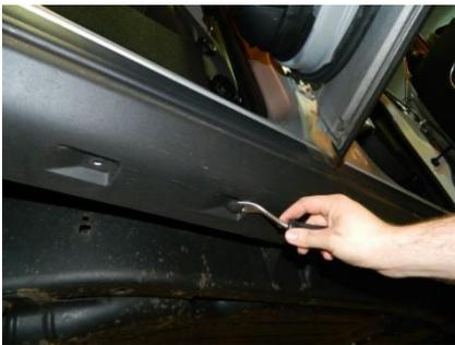
3. Use a trim tool, remove the plastic rivets, then lever the trim outwards, away from the car.
