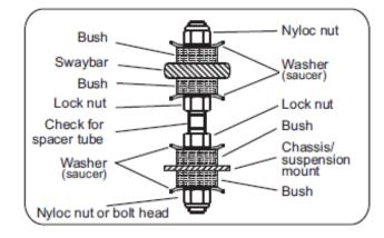
Grease bushing face and ID only Grease bushing ID only
