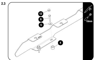
Place a small bead of sealant over each OEM Mounting Point and place a Spacer (Item 4) over each hole. Place a small bead of sealant on the thread of each bolt before fastening.
