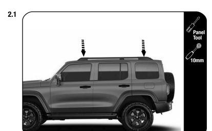
Using a suitable panel tool, remove OEM Roof Rail Covers to reveal the OEM Bolts that fasten the OEM roof rails to the roof of the vehicle.
