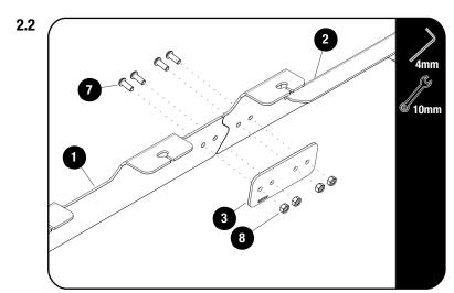
On a flat surface, align a Front Foot Rail (Item 1) and a Rear Foot Rail (Item 2). Place a Joiner Plate (Item 3) over the corresponding holes on the inside of the Foot Rails.
