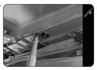
On the inside of the vehicle, place a bead of silicone around each drilled hole.
