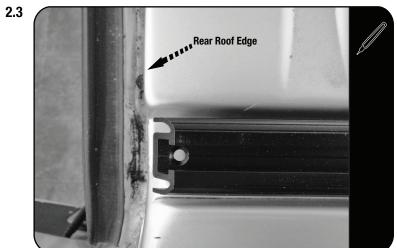
Remove the Roof Lining inside the vehicle.
