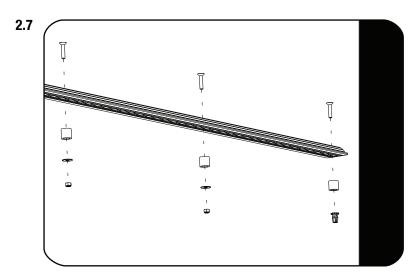
Secure the Tracks to the vehicle using the M6x30 Counter Sink Screws inserted, M6 Large Washers and M6 Nyloc Nuts.
