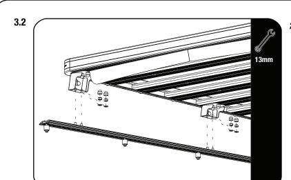
Fit your roof rack to the Tracks using the Stud Plates, M8 x 16 x 1.6SS Flat Washers and M8 Nyloc Nuts shown.
