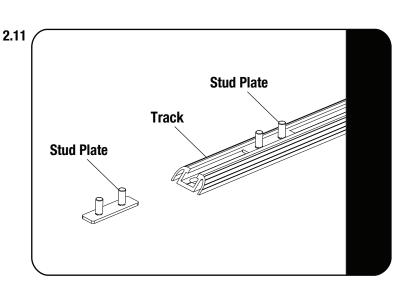
Before placing the rack onto the vehicle, slide two Stud Plates into each track in the approximate position where the Feet will rest on the tracks.
