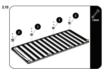
Loosley fit the two Foot Sets - 60mm 70mm (Item 2) to the front and rear slats as shown.
