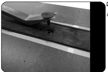
Remove the plastic inserts from the factory mounting points as shown.
