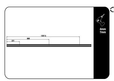
Mark the centres on both the tracks 221mm, 800mm and 1357.5mm from the front as shown. Align the center mounting point on the roof with the 800mm mark you made to ensure the roof mounting points are aligining with the marks you made.
