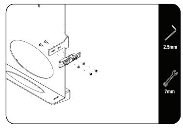
If "needed" adjust the Latch using two M4 x 10 Button head, two M4 Flat Washers and two M4 Nyloc Nuts so that it accomodates your Jerry Can.
