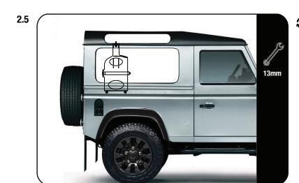
Fully tighten the gutter clamp bracket that was loosened in 2.1
