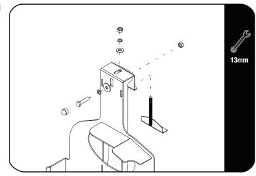
Loosen the fixings that hold the gutter clamp to the Jerry Can Holder so that it can be adjustable when placed on the vehicle.
