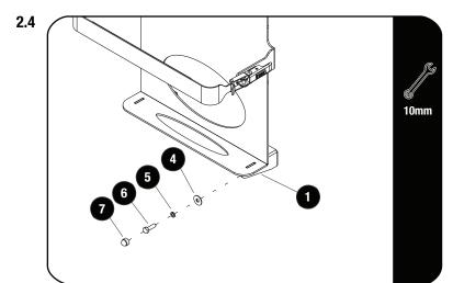
Mount the Vertical Jerry Can Holder (Item 1) to the vehicle using two M6 x 20 Hex Bolts, two M6 Spring Washers and two M6 Flat Washers (Items 6, 5 & 4).
