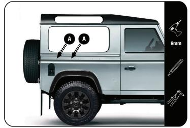
Place the Vertical Jerry Can Holder (Item 1) on the side of the vehicle so that it fits over the top gutter and lines up with the two rivets (Item A) on the vehicle body as shown in 2.3.
