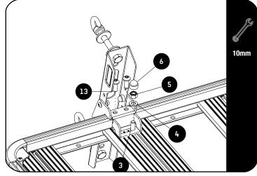
Ensure that one of the MAXTRAX Mount Brackets are aligned with a slat.
