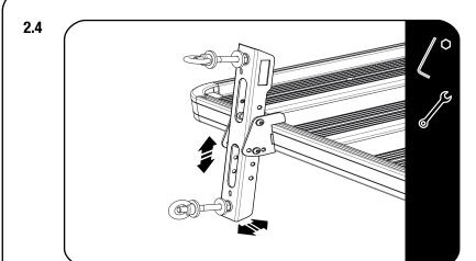
Check the clearance with vehicle body and doors using a MAXTRAX resting on the bracket bolts.
