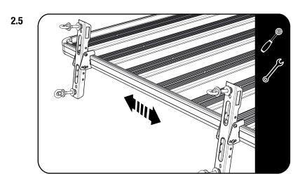
Set final position with a MAXTRAX mounted onto the brackets and fully tighten brackets.
