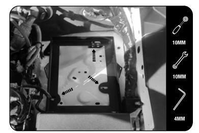
Place the battery bracket bottom frame in the engine bay as shown. Align the 3 holes with the welded nuts in the vehicles body and secure. Refer to 1.1
