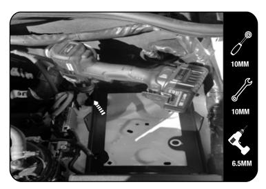
Drill a 6.5mm hole in the vehicle body as shown using the rear corner hole of the bracket as a guide. Secure with fasteners shown in 1.1.
