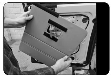
With the latch free, carefully unclip the door panel and remove by feeding the latch back through the panel cut-out.
