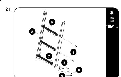
Assemble the left and right ladder sides (Item 2) together with the ladder steps (Item 5) using the M6 x 25 Thread forming Screw (Item 9) as shown.
