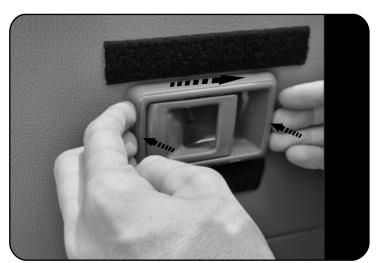
Push the latch forward to release and then to the right to unhook the latch from the door panel.
