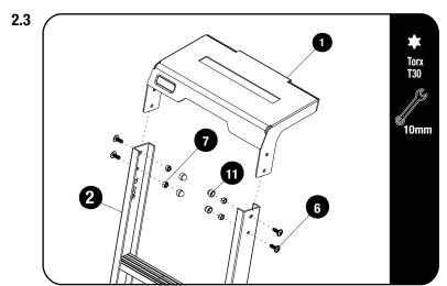
Assemble the top Mount Bracet (Item 1) to the Ladder sides (Item 2) using M6 x 16 Button Head Flange Bolts , M6 Nyloc Nut and M6 Nut Cap (Iten 6 , 7 & 11) shown.
