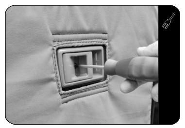
Open the vehicle left hand rear door. Loosen and remove the screw securing the latch to the inside of the rear door using a Phillips Screw Driver.
