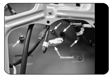
To Remove the number Plate light peel back the plastic cover to expose the wiring and door fasteners.
