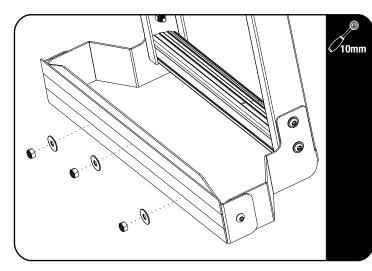
Line up the holes in the Bottom Support (Item 7) with the holes in the door. Refit the light unit pushing the threaded studs through the holes in the Support Bracket, through the door. Loosely secure the light unit using three M6 Large Flat Washers (Item 4) and the OEM nuts previously
