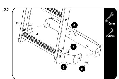
Assemble the Bottom Mount (Item 4) to the side support Bracket (Item 3) Using the M6 x 12 Button head Bolt and Nyloc Nut (Item 7 & 8)
