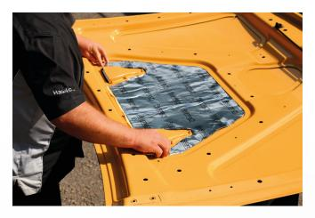
9. Remove the rest of the backing if happy with placement and tack into place. Do not fully press into position, as minor adjustments may need to be made.
