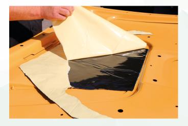
10. Once satisfied, hand press into position and press firmly into recesses.
