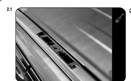
Using a suitable panel tool, start by removing the OEM Mounting Point Covers, to reveal the Mounting Holes on both the left - and right hand sides.
