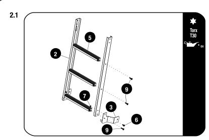
Assemble the left and right ladder sides (Item 2) together with the ladder steps (Item 5) using the M6 x 25 Thread forming Screw (Item 9) as shown.
