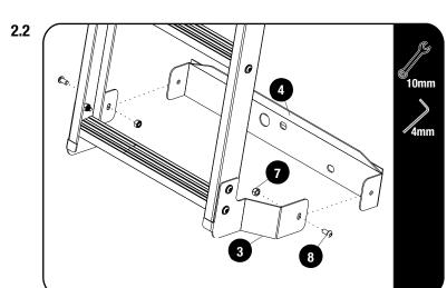
Assemble the Bottom Mount (Item 4) to the side support Bracket (Item 3) Using the M6 x 12 Button head Bolt and Nyloc Nut (Item 7 & 8)
