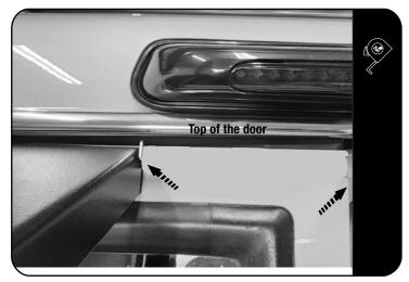
Pull the rubber door seal at the top of the inside door away from the door. Hook the top of the ladder over the top of the door. The middle lip must go between the vehicle door and the rubber door seal and the two side tabs on the outside of the door.
