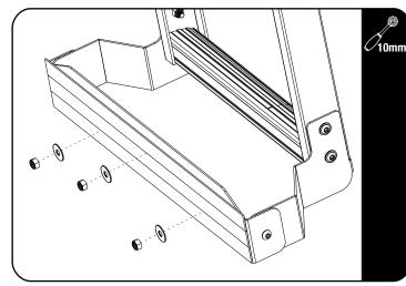
Line up the holes in the Bottom Support (Item 7) with the holes in the door. Refit the light unit pushing the threaded studs through the holes in the Support Bracket, through the door. Loosely secure the light unit using three M6 Large Flat Washers (Item 4) and the OEM nuts previously
