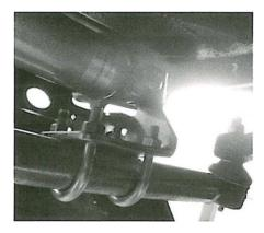
Turn steering fully to the right. Position the bar bracket to allow the damper to be fully extended and rotate for the least resistance to the bushes on the damper. Once positioned securely tighten all nuts which have been left loose. If using a Terrafirma return to Centre steering damper follow the instructions supplied with it on how to set the RTC spring.
