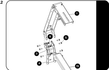
Assemble the Pro Bed Leg (Item 1) to the Front Mounting Brackets (Item 4) and the Front Horizontal Brace and Front Gusset (Item 3 & 15) using M8 x 20 button Head screws and M8 Nyloc Nuts (Item 5 & 6).
