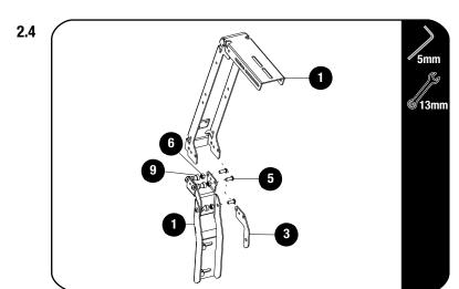
Assemble the Pro Bed Rack Leg (Item 1) to the rear main bracket (Item 1) using the gusset (item 3) and M8x20 Button head screw and M8 nyloc Nut (Item 5 & 6) as shown and fully tighten all the bolts.
