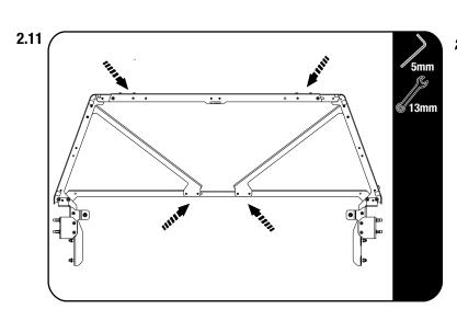
Using clamps and a spirit level clamp the spirit level to the inside of the Front Center Brace and Tighten the M6x20 Button head screws and M6 Nyloc Nuts fitted in 2.3.
