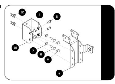
Place the LH & RH Front mounting brackets on the bed ledge and up against the front bed wall. Mark the two side mounting holes and one forward hole per bracket
