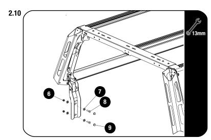
Position the Pro Bed assembly onto the load bed and push it forward until the front mounts are up against the front of the bed and side holes aligned with the plus nuts installed.
