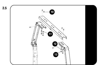
Loosely assemble the rear top truss using the M8x20 Button head screws, M8x19x2 Flat washer and M8 Nyloc Nuts (Item 10,11&12).
