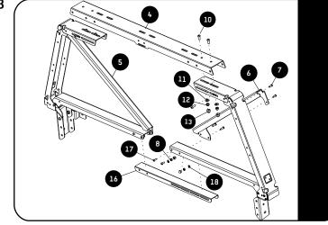
Assemble the Pro Bed Leg (Item 1) and the Gussets (Item3) to the Front Main Bracket (Item 4) using M8x20 Button head screw and M8 Nyloc Nut (Item 5 & 6) as shown and M8x20 Button head screw and M8 nyloc Nut (Item 12 & 5).
