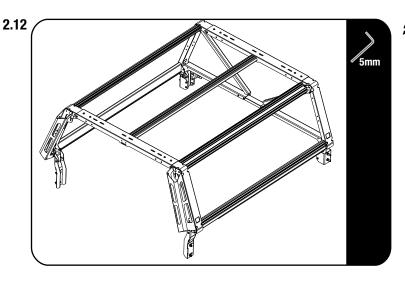
Fully tighten all the bolts and nuts and place nut caps where needed..
