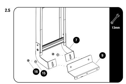
Loosely fit the Base Mount (Item 9) to the Ladder Base ( Item 7) using M8 x 19 x 2 Flat Washer and M8 Nyloc Nut (Items 15 & 16) as shown
