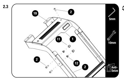
Secure the Ladder Top (Item 1) to the Ladder Top Side Bracket, usings M6 x 20 Button Head Bolts (Item 2), before securing this assembly to the Ladder Side (Item 3) using M6 x 16 Button Head Bolts and M6 Nyloc Nuts (Items 2 & 12) as shown.
