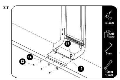
Mark the holes in the Ladder Base Mount onto the bottom lip of the vehicles side
