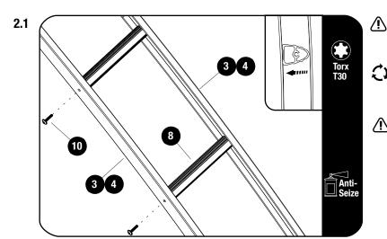
Apply a little Anti seize/oil on screw threads before inserting.
