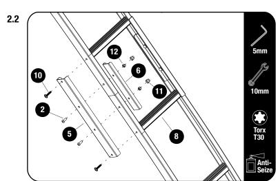
Join the Ladder Top and Bottom assemblies using the Outer and Inner Joiner Channels (Items 5 & 6). Secure using M6 x 16 Button head bolts with M6 Nyloc Nuts (Items 2 & 12) in the center.
