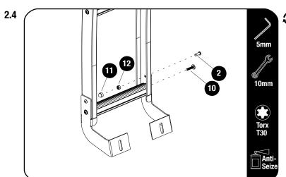
Loosely secure the Ladder Base (Item 7) to the bottom assembly of the ladder, usings M6 x 16 Button Head Bolts and M6 Nyloc Nuts (Items 11 & 12) as shown.
