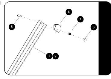
Assemble the Ladder Feet (Item4) to the ends of the Ladder Side Top and Bottom (Items 1 & 2) using M6 x 20 Button Head Bolts and M6 Nyloc Nuts (Items 5 & 7).
