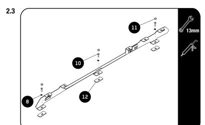
Put a small amount of silicone ove each Mounting Point and place the spacer (Item 12) on top of the silicone, lining up with the hole in the spacer with the mounting point.
