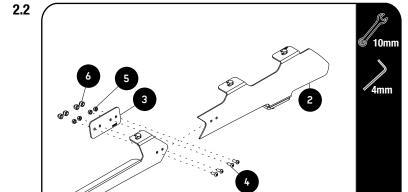
Assemble the Front and Rear foot Rail (Item 1 & 2) together with the Joiner plate (Ietm 3) Using the M6 x 16 Button head screw and M6 Nyloc Nut (Item 4 & 5)
