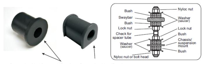
Grease bushing face and ID only Grease bushing ID only
