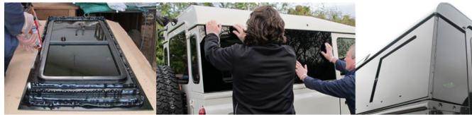
You may require an assistant to help you to carry the glass to your vehicle and bond it. The primer and adhesive application process should be done within 10-15 minutes and immediately after carefully carry the window to the vehicle and press it firmly into position.
