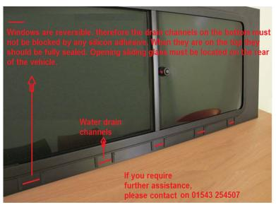
Please be aware that these windows are reversible, therefore the drain channels on the bottom must not be blocked by any silicon adhesive. The drain channels on the top must, however, be fully sealed. The opening sliding glass must be located on the rear of the vehicle as the picture of our Zeppelin windows below demonstrates.
