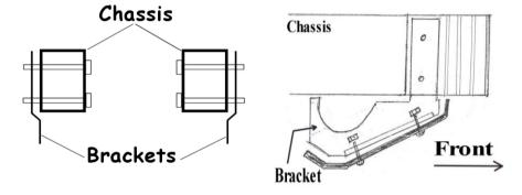
Now bolt the aluminium plate onto the brackets using the bolts provided. Check all nuts and bolts are secure before driving.
