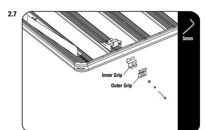
Loosley fit one Inner Grip and one Outer Grip to each Grab On Foot using a M5 Cap Screw, M6 Spring Washer and M6 Cap Screw Washer removed.
