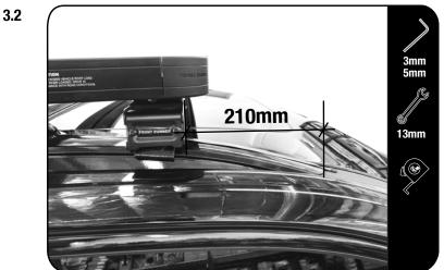
Place your Tray on the vehicle positioning all the feet so that they rest on top of the roof rails.
