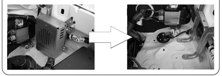
Remove the Speaker Mounting Bracket and Cut the Switch off 45mm from the end as shown.
