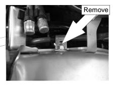
( **B** ) From inside the left wheel arch insert one of the M6 x25 Hex Bolts and one M6 x19 Flat Washer (Items 5 & 10) through the bolt hole in the vehicles body from Step 2A.
