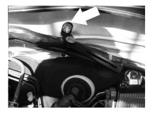
Hook the two J-Bolts (Item9) onto the Battery Bracket. Place the battery in position. Fit the Battery Strap (Item 14, stud side to the rear of the vehicle) over the battery, feeding the two J-bolts through the holes in the Battery Strap and fasten using the two M6 Hex Nuts, two M6 Spring Washers and two M6 x19 Flat Washers (Items 5, 7, 8).
