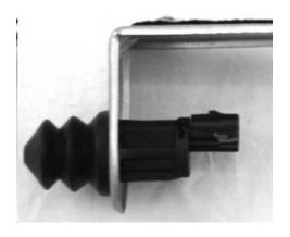
Wet/paint the tip of the Stud protruding from the vehicle's body with a white marker. Press the Switch and Bracket up into position against the Rubber Seal and Stud as shown, marking the position of the Stud onto the back of the Bracket. Drill a 6.5mm hole in the Bracket on your mark.
