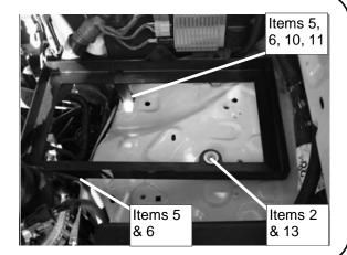
( **B** ) Pull the wiring harness free from the stud in the vehicle's firewall and loosely fasten the Support Bracket assembled in Step 2D to the stud using a M6 x19 Flat Washer and M6 Nyloc Nut (Items 5 &6).
