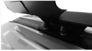
( **F** ) Secure the front Spacers to the vehicle using the remaining M8 x 40 Hex Bolts, M8 Spring Washer and M8 x 19 Flat Washers. Place a M8 Nut Cap (Item 1) over each Bolt Head once fastened.
