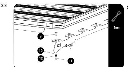
Fit your Tray to the Foot Rails using M8 x 20 Hex Bolts, M8 x 16 x 1.6 Flat Washers and M8 Nyloc Nuts (Items 9, 10 & 12) as shown.
