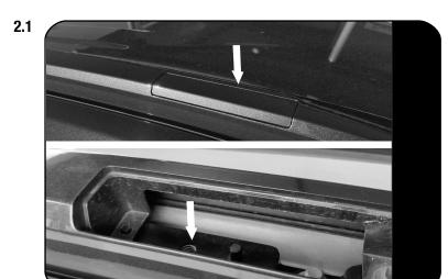
Start by removing the covers on the roof trim, using a trim removal tool. Do this for the front and rear, to reveal the OEM mounting points.
