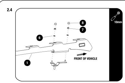
Place the Foot Rails (Item 1) over the corresponding studs on each Saddle Bracket as assembled in Steps 2.2 and 2.3.
