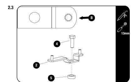
At the rear of the vehicle, place a Spacer (Item 5) over each Mounting Hole.
