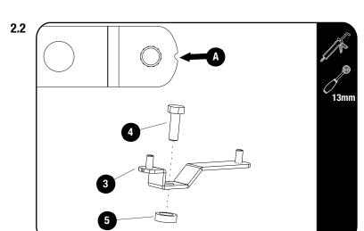
Starting at the front of the vehicle, place a Spacer (Item 5) over each Mounting Hole.
