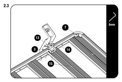
Choose a suitable location for the ladder. See 2.4 for positioning. Leave 2 slats open between the two Holder assemblies.
