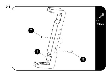
Secure M8 x 35 Hex Bolts (Item 12) to each of the Holders (Item1) using M8 Nyloc Nuts (Item 7) as shown.
