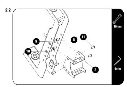
Assemble the Rack Mount (Item 2) To the Holder (Item 1) using M6 x 16 Button Head Bolts, M6 Nylon Washers and M6 Nyloc Nuts (Items 8, 10 & 11).
