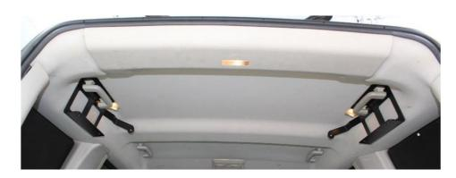
Open one of the passenger side doors, slide the rack in to the back of vehicle then lift the rack up and slide in to place so that it rests on the mounting brackets. This may be easier with an assistant but is not necessary.
