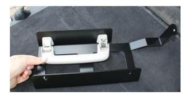
Offer the grab handles and brackets up to their original location before using the panhead retaining screws to secure them in place on both sides of the vehicle.
