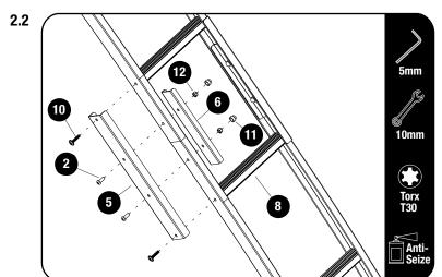
Join the Ladder Top and Bottom using the Outer and Inner Joiner Channels,
