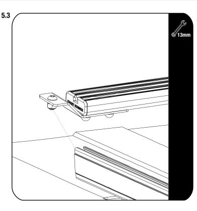
The Slat Z brackets can be inverted as shown if you wish to have the rack lower on your vehicle.
