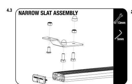
Loosely assemble the Slat Z Brackets (Item 2) to the Narrow Slats using M8 x 20 Hex Bolts and M8 Nyloc Nuts.
