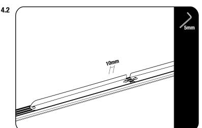
Center the Wind Deflector on the rack and move the bolt assemblies from fig 4.1 into the slots as shown in fig 4.2.
