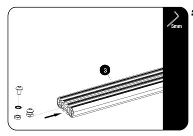
Insert two Button Head Bolts, M8 Half Nuts and M8 Schnorr Washers assemblies into the Narrow Slat as shown. Slide them to the center of the Narrow Slat (Item 3), making sure that the Schorr Washer is above the T-Slot Channel.
