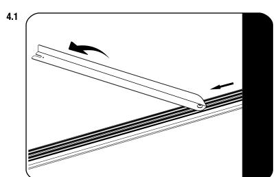
Slide the nut assembled to the Wind Deflector into the T-slot of the Narrow Slat as shown.
