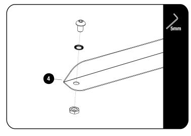
Loosely assemble the M8 x 12 Button Head Bolt, M8 Schnorr Washers and M8 Thin Nut both LH & RH Wind Deflectors (Item 4) as
