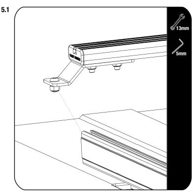
Slide pre assembled Slats into the Side Profiles. Space the Slats at 404mm increments, or at your chosen spacing. These can be adjusted at any stage.
