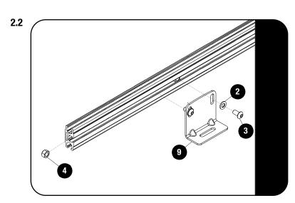
Loosely assemble the VW Crafter Feet (Item 9) using M8 x 16 Button Head Bolts, M8 Flat Washers and M8 Nyloc Nuts and slide them into the side profiles. They must still slide freely.
