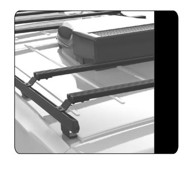
If a roof A/C is fitted to the vehicle space the slats around the A/C at 202mm increments on shorter lengths and 404mm on the longer lengths
