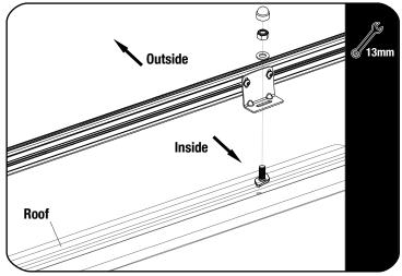
Place pre-assembled Side Profiles over the mounting points. Align feet with factory holes and secure the feet to the roof using M8 x 25 T-Bolts, M8 x 16 Flat Washers, and M8 Nyloc Nuts. You will need a friend to help. Fully tighten.
