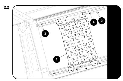
Loosley fit the Molle Panel (Item 1) to the M8 Thin Nuts (Item 3) that was inserted in 2.1 using the M8 x 16 Button Head Screws and M8 Schnorr Washer (Item 2 & 4).DO NOT FULLY TIGHTEN.
