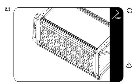
Once all 4 Molle Panels are in place fully tighten the M8 x 16 Button Head screws.
