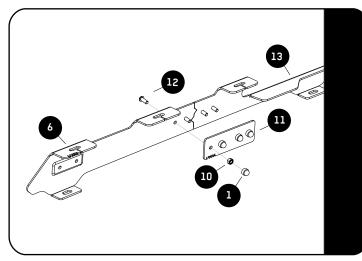
Loosely join the Front and Rear Foot Rails (Items 6 & 13) together using M6 x 16 Button Head Bolts, M6 Nyloc Nuts and the Joiner Plate (Items 10, 11 & 12) as shown.
