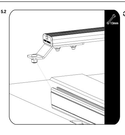
Slide pre-assembled Slats into the Side Profiles as shown. Space the Slats at 404mm increments, or at your chosen spacing. These can be adjusted at any stage.
