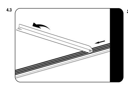
Slide the nut assembled to the Wind Deflector into the T-slot of the Narrow Slat as shown.
