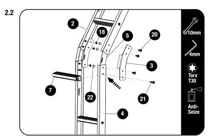
Apply a little Anti Seize / oil on Thread Forming Screws before inserting. Note these are thread forming screws.
