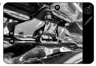
Loosen and remove the Left Hand OEM Hinge Bolts to fit the Top Mounting Bracket (Item 23) to act as a guide for the placement of the ladder.
