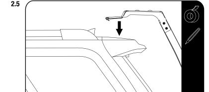
With the hatch closed place the ladder onto the top of the hatch. Hold firmly in place to prevent it moving and open the hatch to shift and align with holes in top mount brackets.
