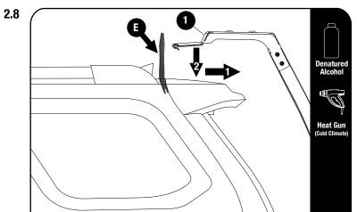
Clean the top area of the hatch with Denatured Alcohol.
