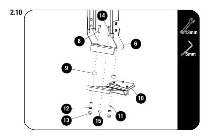
Secure the Ladder assembly to the Bottom Clamp (Item 10) as shown.
