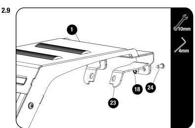
Secure the Top Step Bracket (Item 1) to the two Top Mounting Brackets (Item 23) using M6 x 12 Button Head Bolts and M6 Nyloc Nuts (Items 24 & 18)
