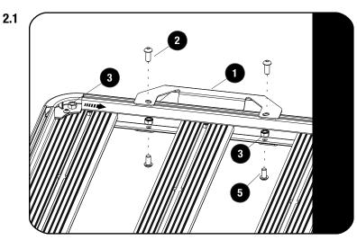
Secure the Handle Light Rack Bracket (Item 1) to your Roof Rack using M8x16 Button Heads, M8x20 Button Heads, M8x16x1.6 Flat Washers and M8 Nyloc Nuts (Items 2,3 & 5).
