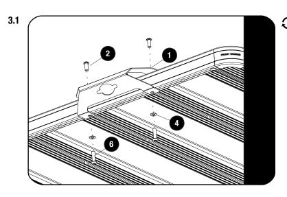
Secure the Handle Light Rack Bracket (Item 1) to your Roof Rack using M8x16 Button Heads, M8x30 Button Heads, M8x16x1.6 Flat Washers and M8 Nyloc Nuts (Items 2,3 & 6).
