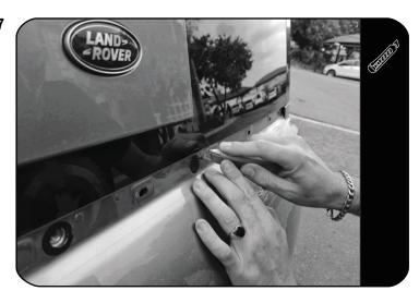
Remove Sealing Patch that is located behind the plastic trim shown in Fig 2.6.
