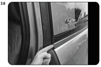
Remove the Plastic Trim by using a Plastic Panel Tool or similar.
