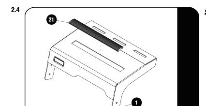
Inset the Rubber Step (Item 22) into the ladder Top Hat (Item 1), cut off the excess rubber if there is any.
