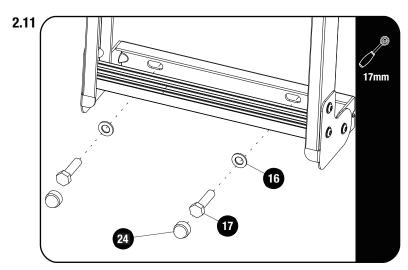
Secure your Ladder to your vehicle using M10 x 40 Hex Bolt and M10 Flat Washer (Items 16 & 17).
