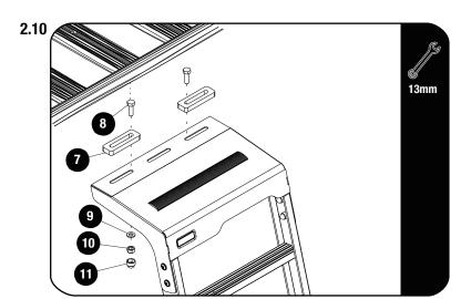
Using the bottom holes as reference, choose the corresponding roof rack slats.
