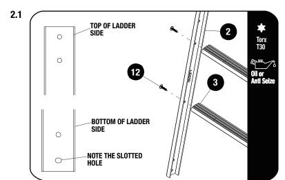
Assemble the Ladder Rungs (Item 3) to the Ladder Sides (Items 2) using M6 x 25 Thread Forming Screws (Item 12) as shown.
