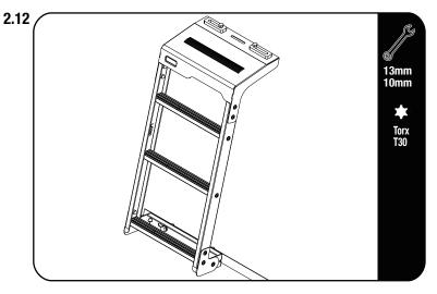
Tighten all the bolts and nuts and the put Nutcaps on all the nyloc Nuts (Items 11 & 6)
