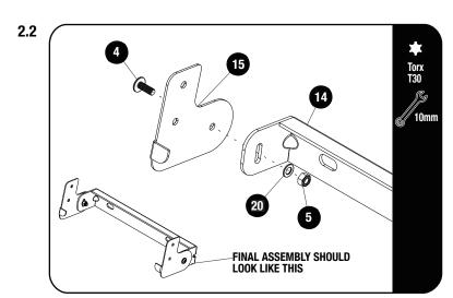
Loosely assemble the Bottom Bracket (Item 14) to the Bottom Bracket Sides (Item 13 &15) using the M6 x 12 Flanged Button Head Screws (Item 4) and M6 Nyloc Nuts (Item 5)
