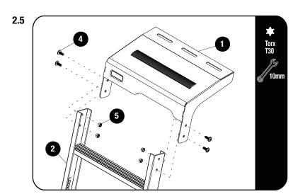
Loosely assemble the Ladder Top (Item 1) to theLadder Sides (Item 2) using M6 x 16 Flanged Button Head Screws and M6 Nyloc Nuts (Items 4 & 5) as shown.
